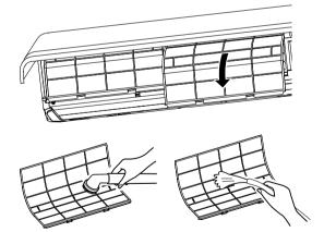
Insert the upper portion of air filter confirming to fit its right and left edges on the indoor unit until it is firmly set.
