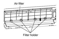
Use a vacuum cleaner to remove the dust from the filters or wash them with water.If you wash the air filters, dry them in the shade.
